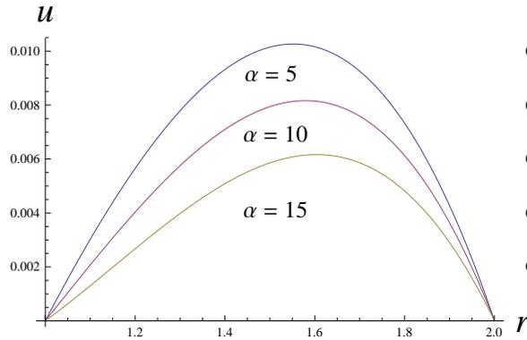
Fig. 6: Velocity profiles for permeability variation  $k = k_0 r^2$  when  $q = 2$ ,  $M = 10$  for different values of  $\alpha$ .
