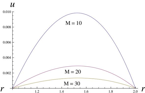
Fig. 5: Velocity profiles for permeability variation  $k = k_0 r$  when  $q = 2$  and  $\alpha = 5$  for different values of  $M$ .
