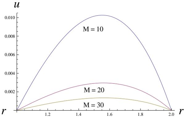
Fig. 7: Velocity profiles for permeability variation  $k = k_0 r^2$  when  $q = 2$  and  $\alpha = 5$  for different values of  $M$ .
