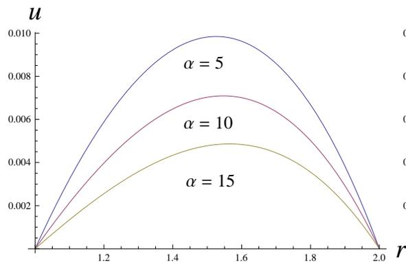
Fig. 4: Velocity profiles for permeability variation  $k = k_0 r$  when  $q = 2$ ,  $M = 10$  for different values of  $\alpha$ .
