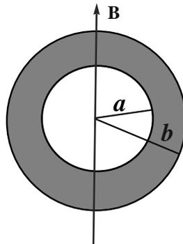
Fig. 1: Cross-section of annular tube filled with porous medium with transverse applied magnetic field.
