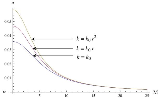
Fig. 9: Variation of velocity with  $M$  for different cases of permeability variation when  $\alpha = 5$ ,  $q = 2$  and  $r = 1.5$ .
