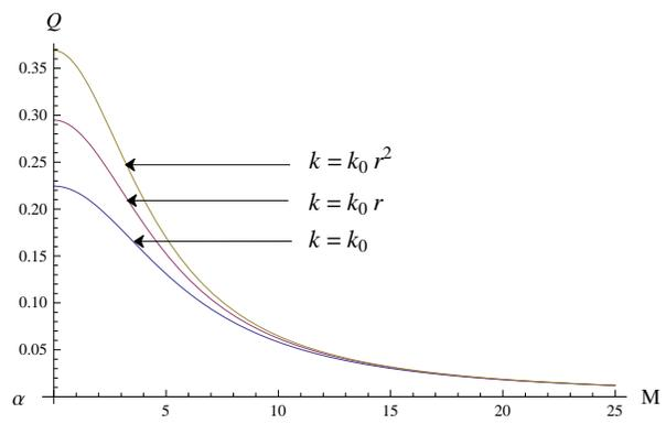
Fig. 11: Variation of rate of volume flow with  $M$  for different cases of permeability variation when  $\alpha = 5$  and  $q = 2$ .
