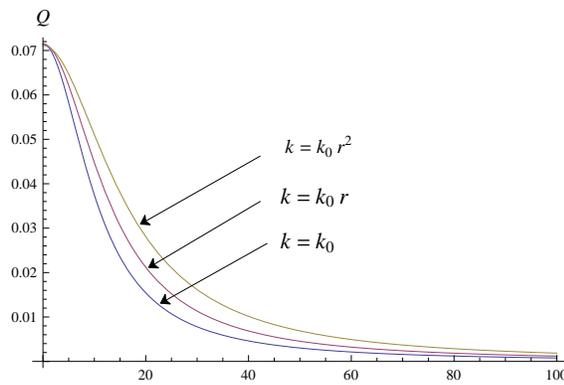
Fig. 10: Variation of rate of volume flow with  $\alpha$  for different cases of permeability variation when  $M = 10$  and  $q = 2$ .
