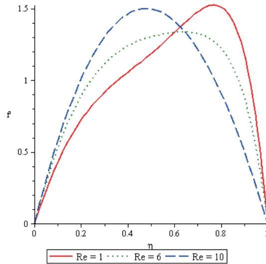
Fig. 2: Plot of  $f'(\eta)$  v/s  $\eta$  at  $S = 0.1$  for different values of Reynolds number (Re).
