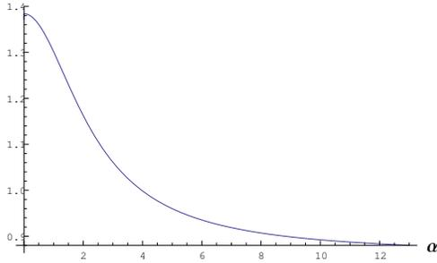
Fig. 7: Variation of volume flow rate with  $\alpha$  for Couette-Poiseuille flow when  $q = 2$  and  $\beta = 15$ .
