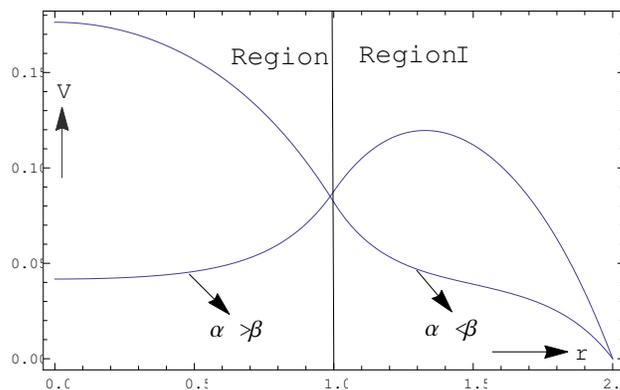
Fig. 2: Variation of velocity for poiseuille flow with radial distance  $r$  for two different cases, when  $\alpha > \beta$  ( $\alpha = 5$  and  $\beta = 2$ ) and when  $\alpha < \beta$  ( $\alpha = 2$  and  $\beta = 5$ ) for fixed  $q = 2$ .
