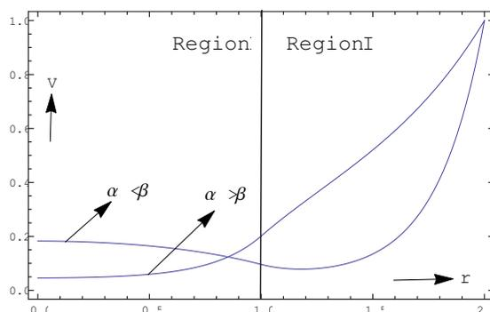
Fig. 6: Variation of velocity for Couette-Poiseuille flow with radial distance  $r$  for two different cases, when  $\alpha > \beta$  ( $\alpha = 5$  and  $\beta = 2$ ) and when  $\alpha < \beta$  ( $\alpha = 2$  and  $\beta = 5$ ) for fixed  $q = 2$
