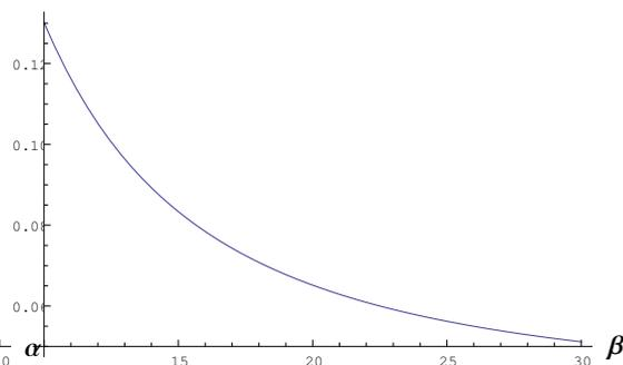
Fig. 4: Variation of volume flow rate with  $\beta$  for Poiseuille flow when  $q = 2$  and  $\alpha = 8$ .
