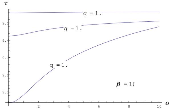
Fig. 9: Variation of shear stress for Couette - Poiseuille flow on the impermeable surface of cylinder with  $\alpha$  for different values of gap parameter  $q$  and fixed value of permeability parameter  $\beta = 10$ .
