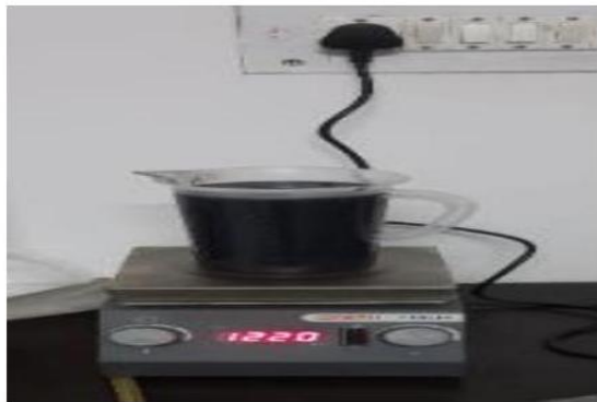
Figure 3 magnetic stirrer process for fuel preparation.
